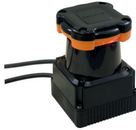
Fig. 5. UTM-30LX laser range finder from HOKUYO.
